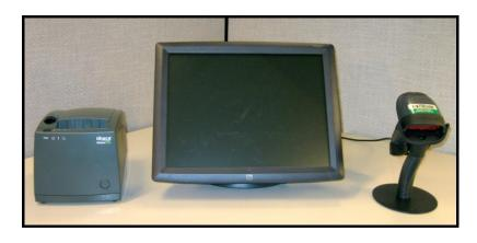
The terminals are computer based and should only be used in climate-controlled environments. They should not be exposed to high temperature, high humidity, excessive dust, rain, or splashing liquids. Placing the terminal near a deep fryer or source of heat will lead to premature failure.
