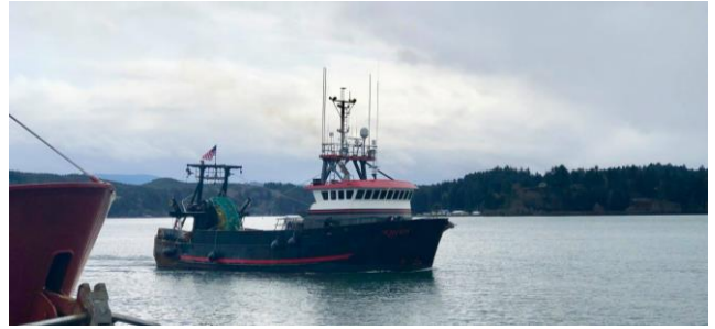
Groundfish trawlers are the largest fishing vessels and can be identified by their large net reels.
