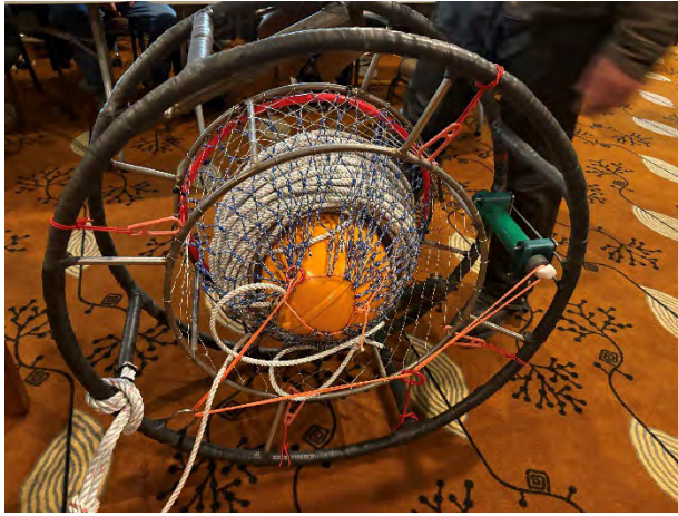
The Guardian Ropeless system line containment sled, using a crab pot frame, shown tipped vertically (left) and how it would be deployed to the seafloor (right).
