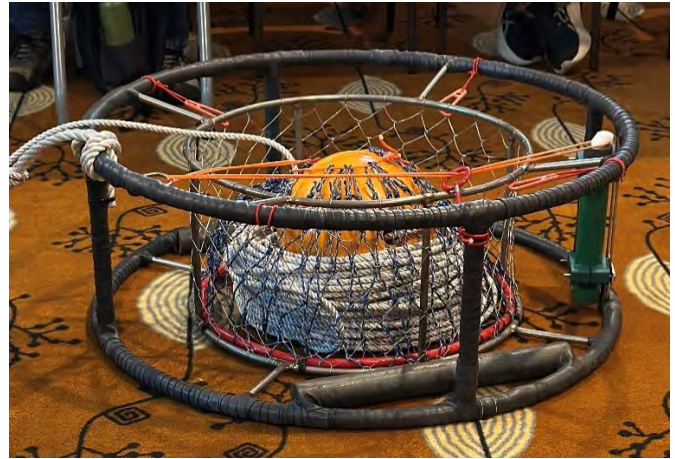
The Guardian Ropeless system line containment sled, using a crab pot frame, shown tipped vertically (left) and how it would be deployed to the seafloor (right).
