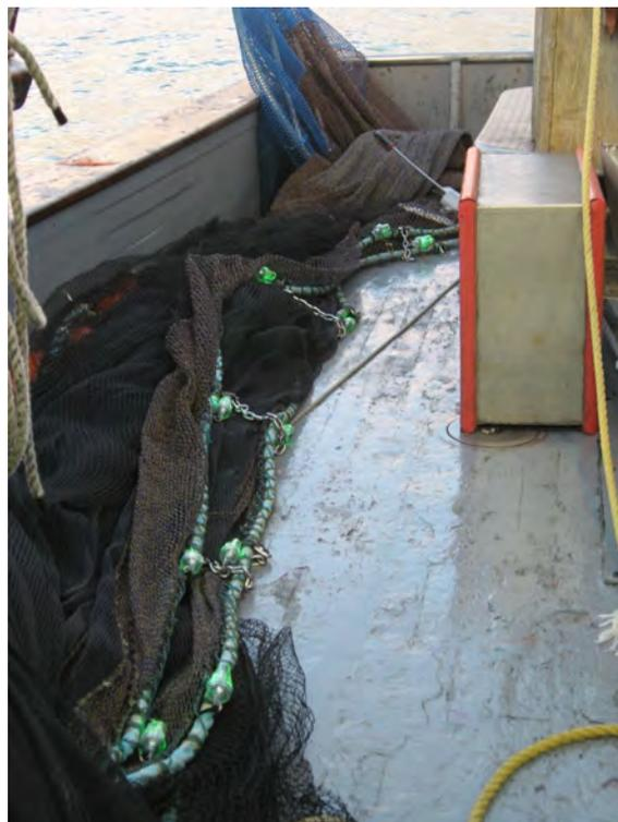
**Figure 17. Photo of the port-side net on deck with ten green lights attached to the fishing line (as tested). The rigid-grate BRD is shown leaning at the stern. The lights proved durable after the nets were dragged on-board at least twice a day, for 8 days.**
