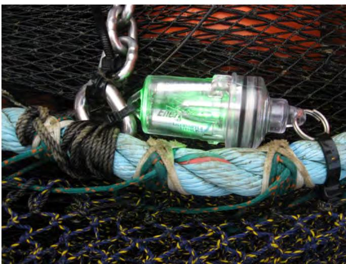
**Figure 18. Photo of a single green Lindgren-Pitman Electralume light zip-tied to the fishing line of a shrimp trawl. We found that looser zip-ties worked better to avoid torquing the light.**
