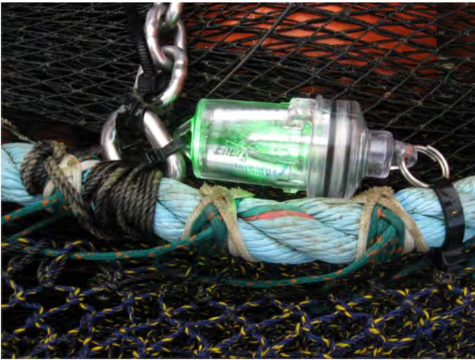
**Figure 2.** Photo of a single green Lindgren-Pitman Electralume light zip-tied to the fishing line of a shrimp trawl. We found that looser zip-ties worked better to avoid torquing the light.
