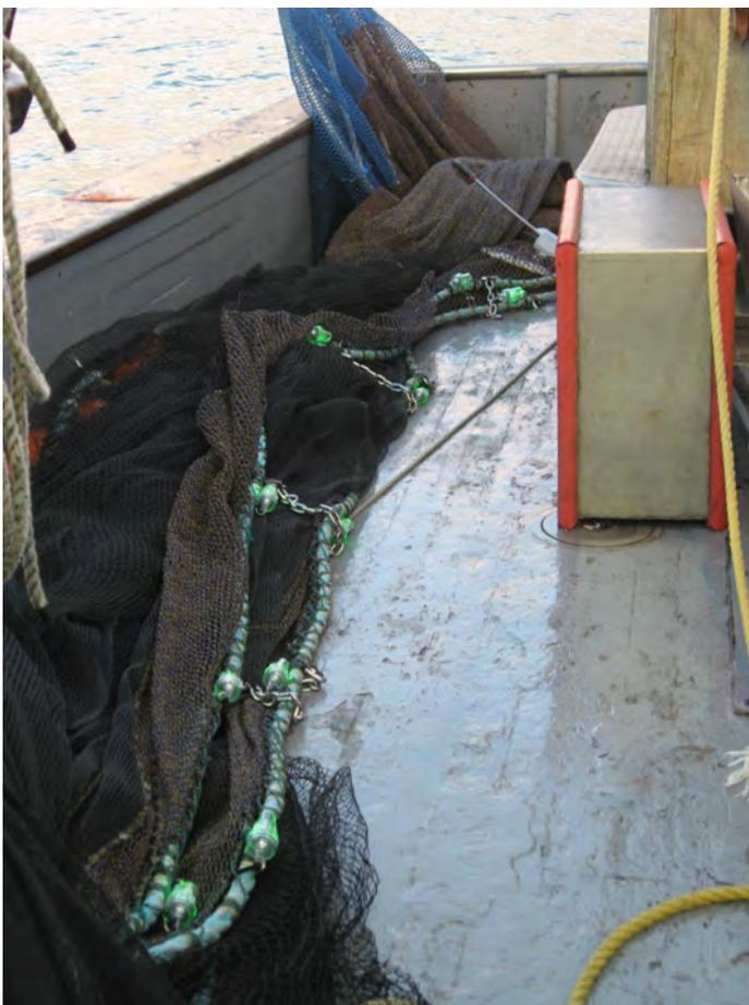
**Figure 4.** Photo of the starboard-side net on-deck with ten green lights attached to the fishing line (as tested). The rigid-grate BRD is shown leaning at the stern. The lights proved durable after the nets were dragged on-board at least twice a day, for 8 days.
