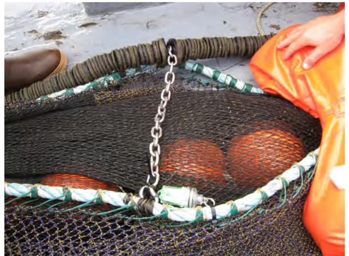
**Figure 3.** The same light shown in Figure 2 showing its relative position to the chain droppers and doughnut-covered groundline. While fishing, the fishing line was about 15 inches above the groundline on each net.
